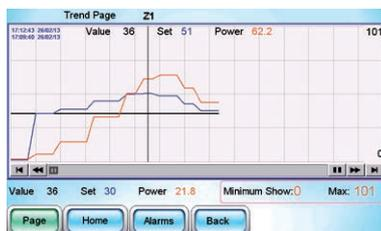
For each loop is available Trend page dedicated to the graphical display of setpoint value and temperature control, view over time. Each square represents 1 minute, then the screen will show every 15 minutes. With 24 loop operating page, includes the graphical display of 4 loops.
