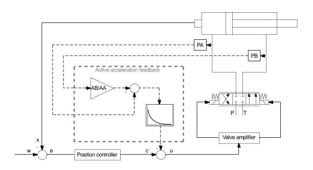
Position control with acceleration feedback via the differential pressure
