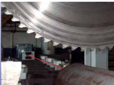
Determination of coil diameter - Coiler
