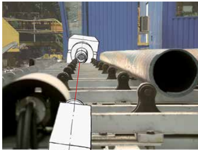
Length measuring of pipelines - transversal transport
