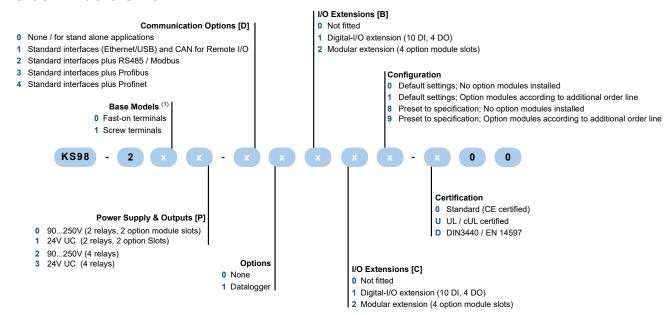
(1) Universal Input, 2 digital Inputs, TPS, 2 option module slots
