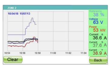
• Current: wih REVO M 1PH and REVO CL the avarage value measured on the single phase units is displayed. With REVO M 2-3PH again only one avarage is an avarage value of the three phase. With REVO E and Multidriv -3PH N°3 avarage current are
