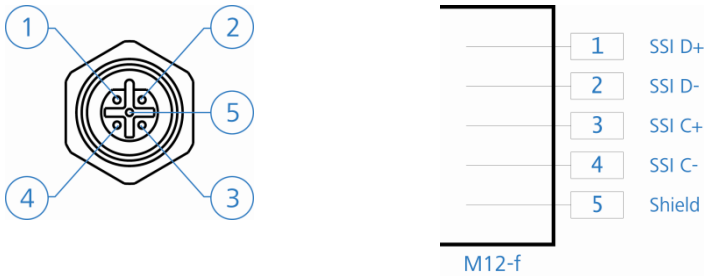
Figure 9 : Connection diagram LDM301S SSI
