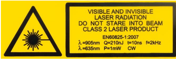
Figure 1 : Device warning sign 1
