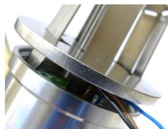
Now the puck without the display can be properly positioned and installed back in the sensor head and the wiring can be reconnected to the cable terminal. Then the large display can be mounted → see "Retrofitting the display if a display was not yet installed".
