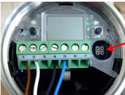
Connection plug for the MPI-200-F adapter as an intermediate plug between the ILM-4 electronics and the MPI-200 connection 3 (see the next figure).
