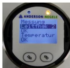
After the sensor is started, the screen saver appears in which the process values of the sensor are displayed one after the other. To reach the start page from here, press one of the two buttons briefly. Further information on operating the display can be found in the quick start manual and in the operating manual for the modular sensors (ILM-4, NSL-F...).
