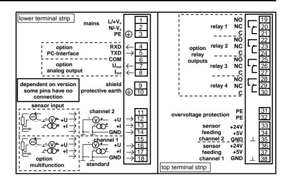
for 0..20 mA, 4..20 mA, 0..10 V, PT-100 or mV-differential signals
