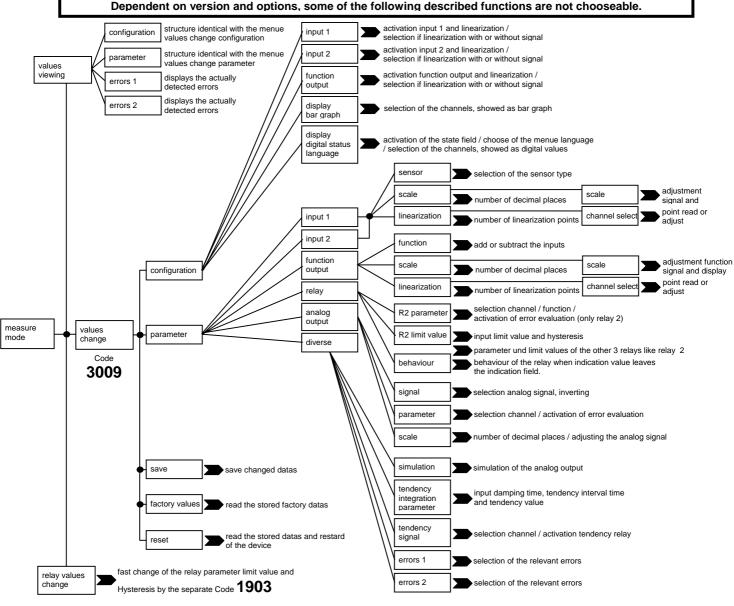
Use the key "OK" to enter the main menue. From here each menue can be selected, using the keys "+" or "-" and entered, using the key "OK". Changings can only be made in the menue structure "values change", but the relay datas also, using the menue "relay values change".
