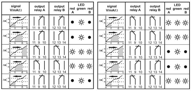
The set limit value A equals the switching value and the limit value B equals the switch back value.
