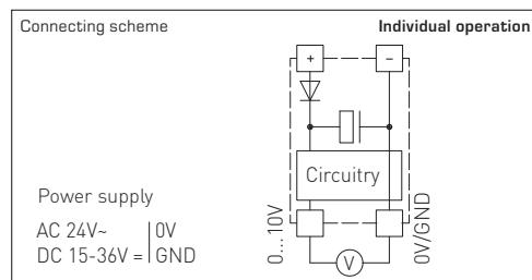
When several devices are supplied by one 24V **AC voltage supply**, it is to be ensured that all "positive" operating voltage input terminals (+) of the field devices are connected with each other and all "negative" operating voltage input terminals (-) (= reference potential) are connected together (in-phase connection of field devices). All outputs of field devices must be referenced to the same potential!
