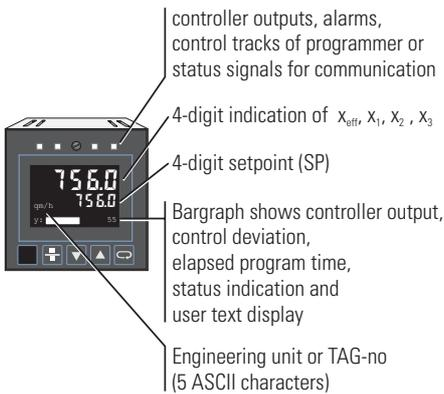
Fig. 3 Programmer with analog output and 4 control outputs
