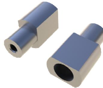
Centering and assembly gauge for centering the base plate on the motor flange or an adapter plate and also positioning the magnet
