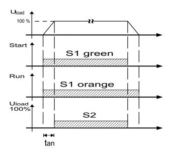
switching function S1 was accomplished (connectors S1 and LED 2 (S1) (orange) are activated at the same time)
