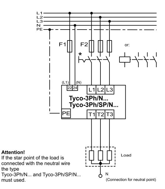
For isolate you can use plug connection, fuses, circuit-breakers, load-breakers and residual current devices (RCDs). Contactor, however, can be used only in exceptional cases and due to isolate.
