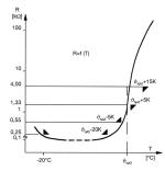
PTC-temperature sensors according to DIN 44081 (triplet design DIN 44082) are used to protect electrical machines against thermal overload. According to the present DIN standard they are arbitrarily exchangeable among themselves. It is a range of types from 60 to 190°C available.
