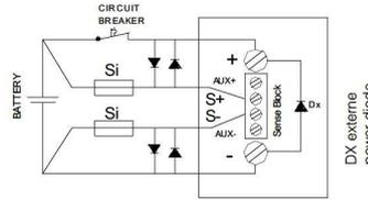
**Remote Sensing (2V per lead load, fig6)**
