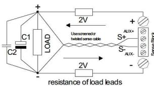
**Remote Sensing (2V per lead load, fig6)**
