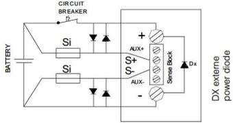
**Remote Sensing (2V per lead load, fig6)**
