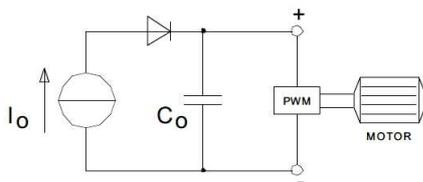
Conventional power supply: breaking power charges output capacitor C<sub>o</sub>
