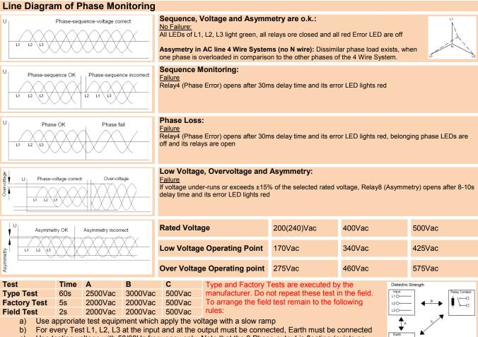
c) Use testing voltage with 50/60Hz frequency only. Note that the 3 Phase output is floating (exists no ohmic reference to Earth)
