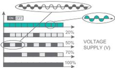
This firing is performed digitally within the thyristor unit at zero volts, producing no EMC interference. Analogue input is necessary for BF and the number of complete cycles must be specified for 50% power demand. This value can be between 1 and 255 complete cycles, determining the speed of firing. When 1 is specified, the firing mode becomes Single Cycle (SC).
