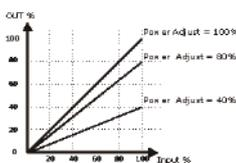
It's a scaling factor of the input command signal and limit the output of Thyristor unit. This parameter can be adjusted from 1 to 99% via RS485 or by the front of the unit. If this parameter is setted at 50% and the input signal is 100% the output become 50%. This feature is very useful to reduce the power when a zone has been oversized or when a temperature controller gives same reference to more unit along a furnace.
