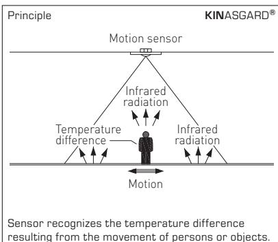
Sensor recognizes the temperature difference resulting from the movement of persons or objects.
