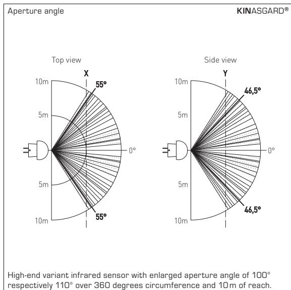
High-end variant infrared sensor with enlarged aperture angle of 100° respectively 110° over 360 degrees circumference and 10m of reach.
