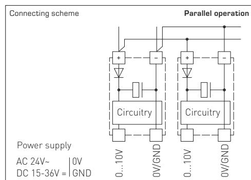
When several devices are supplied by one 24V **AC voltage supply**, it is to be ensured that all "positive" operating voltage input terminals (+) of the field devices are connected with each other and all "negative" operating voltage input terminals (-) (= reference potential) are connected together (in-phase connection of field devices). All outputs of field devices must be referenced to the same potential!
