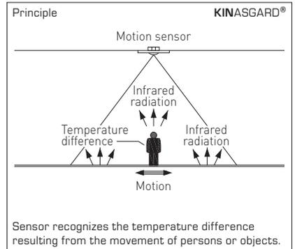
In all KINASGARD® motion sensors and presence detectors, a high-end variant infrared sensor with enlarged angle of aperture is exclusively used.
