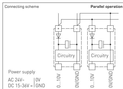
When several devices are supplied by one 24V **AC voltage supply**, it is to be ensured that all "positive" operating voltage input terminals (+) of the field devices are connected with each other and all "negative" operating voltage input terminals (-) (= reference potential) are connected together (in-phase connection of field devices). All outputs of field devices must be referenced to the same potential!
