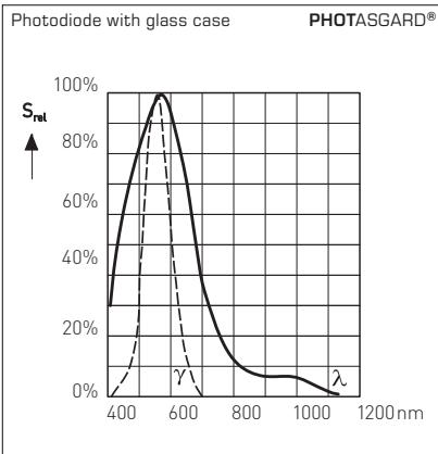
Characteristic curve showing the sensor's sensitivity in respect of the wavelength  $\lambda$  of light. The broken line represents the light perception of the human eye.
