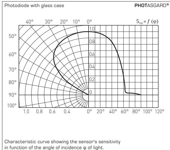
Characteristic curve showing the sensor's sensitivity in function of the angle of incidence  $\varphi$  of light.
